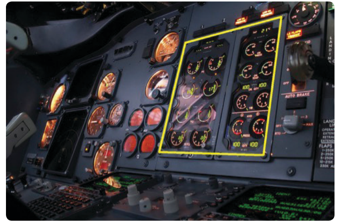
Figure 8-3. Engine instruments centered on the cockpit front instrument panel for easy viewing by both co-pilot and pilot (Boeing 737 aircraft).
