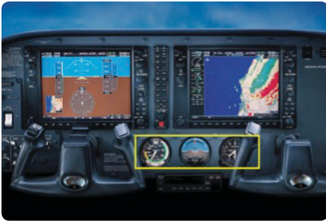
Figure 8-2. Analog instruments embedded in a glass cockpit for redundancy (Cessna Sky Hawk).
