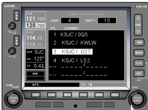
In cursor mode, scroll to the stored flight plan of your choice. 2
