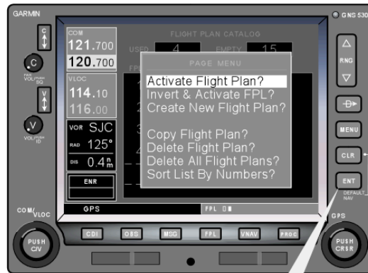
Press the MENU button to display your options, then scroll to the Activate Flight Plan?, and press the ENT button to make your selection. 3
