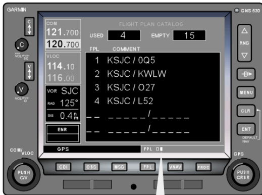
The second extended page of the flight plan page contains the list of stored flight plans. 1
