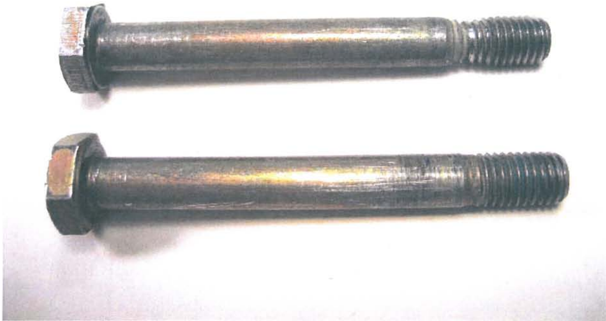
(Shown: stretched tie back bolts from over-torque)
