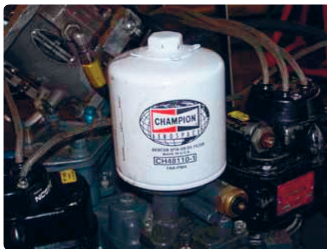
Figure 9-6. Spin-on oil filter.
