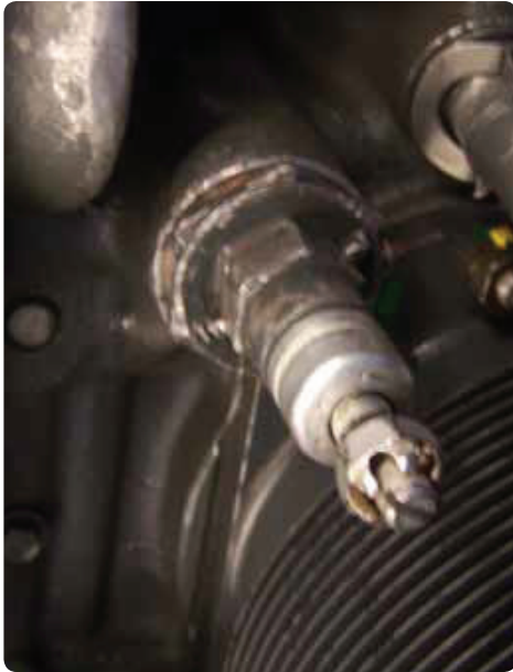
Figure 9-8. Oil pressure relief valve adjustment.
