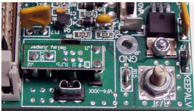
The chief advantage of a master solenoid is the fact that it is generally located very close to the battery. This minimizes the length of the unswitched lead. This is a valuable safety consideration. If the External master solenoid is to be used, the relay K1 should be unplugged and replaced with the relay jumper provided by the manufacturer. (See Figure 8)
