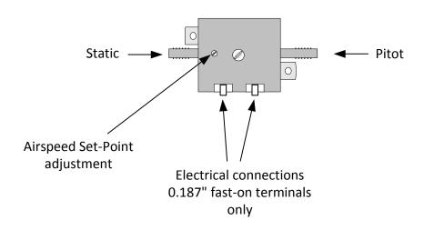
NOTE: Airspeed set-point is adjusted by turning small screw:
