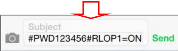
The above message is the “ON” message for outlet 1. You must touch the Send button to transmit the message and turn outlet 1 ON
