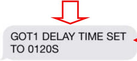
Confirmation of 2 minute RUN time for Outlet 1. If no confirmation is received the change was not made
