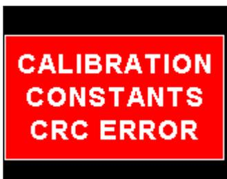
Calibration constants CRC error. The instrument could possibly have a non-volatile memory failure in which case the instrument will then have to be returned to the factory.
