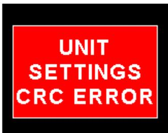
Unit settings CRC error. Load default settings to restore to factory defaults. If the error message still persists then it could possibly be a non-volatile memory failure in which case the instrument will then have to be returned to the factory.
