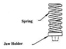
5. Hold tool with the puller shaft pointing down and Jaw Pusher fully extended. Screw the Jaw Holder on to the Puller Shaft. HAND TIGHTEN ONLY.
