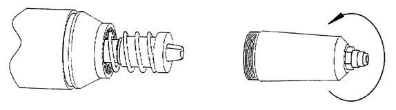
2. Remove the jaw holder by unscrewing it in a counterclockwise direction. Drop jaws out from the spring side. Pump handles (approx. 2-3 times) until jaw pusher is fully extended. Stop pumping handles as soon as the jaw pusher is in extended position.
