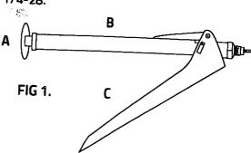
NOT apply excessive force or that threads will be stripped. Release handle (C) and pull knob (A) completely out, this will release pull-up stud from the insert.
