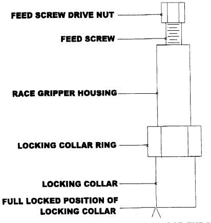
DURING USE LOCKING COLLAR END MUST BE FLUSH WITH RACE GRIPPER TUBE END
