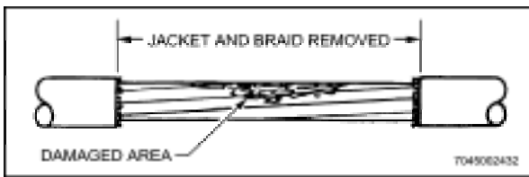
Figure 5-18 Damaged Multi-conductor Cable
