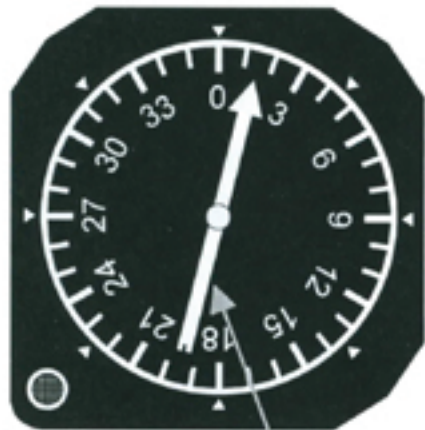
Rotating ADF Needle
