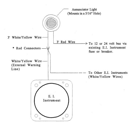
\* Note: When installing the Red Slip-on Connectors double over the wires and double crimp the connectors very tightly. Also, insure the tab is centered in the male connector. If the connectors are disconnected several times the female connector may become loose. If this happens, use a pair of needle nose pliers to retighten the female connector. To protect against corrosion use two drops of oil on the female connector before mating.
