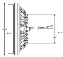
Voltage: 9-40VDC Current: 2.5A at 28VDC Power: 70 Watts
